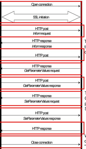
The CPE initiates the connection. The CPE is always the initiator, though the ACS can make a "Connection Request" to stimulate the CPE to initiate a connection. The underlying protocols establish a connection. TR-069 is almost always performed over Secure Socket Layer (SSL), unless for testing purposes.
